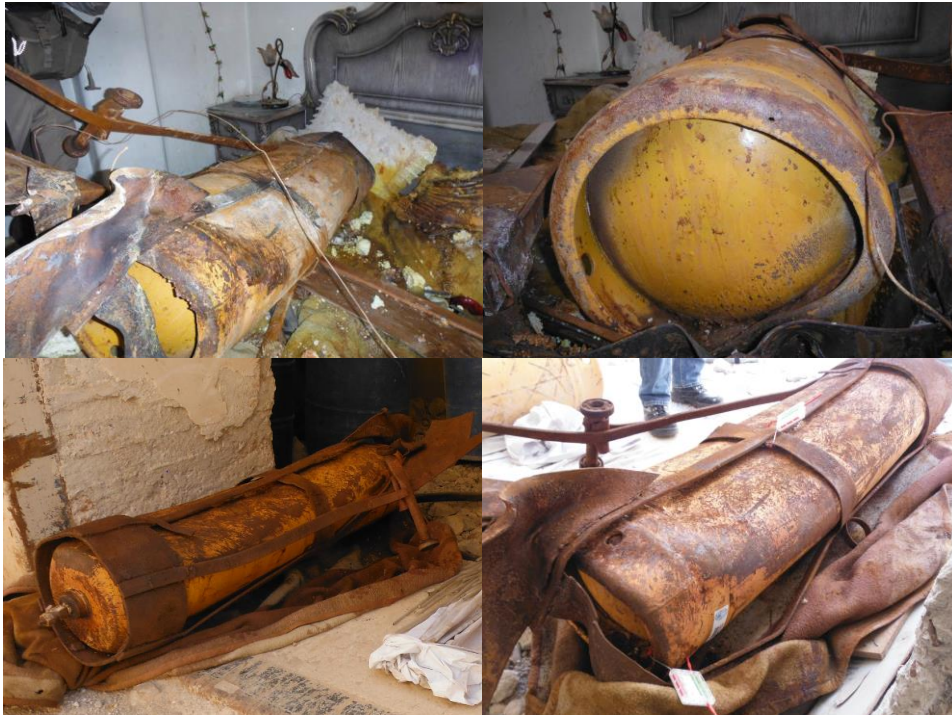
FIGURE 14: DAMAGE OBSERVED ON THE CYLINDER
